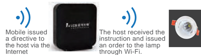
Outdoor long distance remote control schematic
